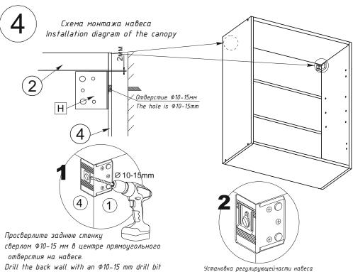
in the center of the rectangular hole on the canopy. Installation of the regulating part of the canopy
